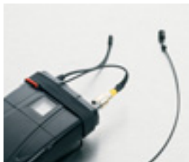
Correct way to wind up the cable of the Miniature Microphone. Please note the slack after the connector.
